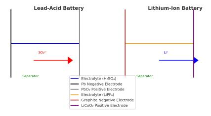
The above schematic compares the structures of lead-acid and lithiumion batteries. Note the differences in electrode materials, electrolyte compositions, and ion transport mechanisms.
